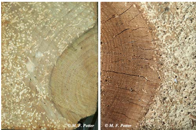
Larvae prefer to tunnel in sapwood more than heartwood.
