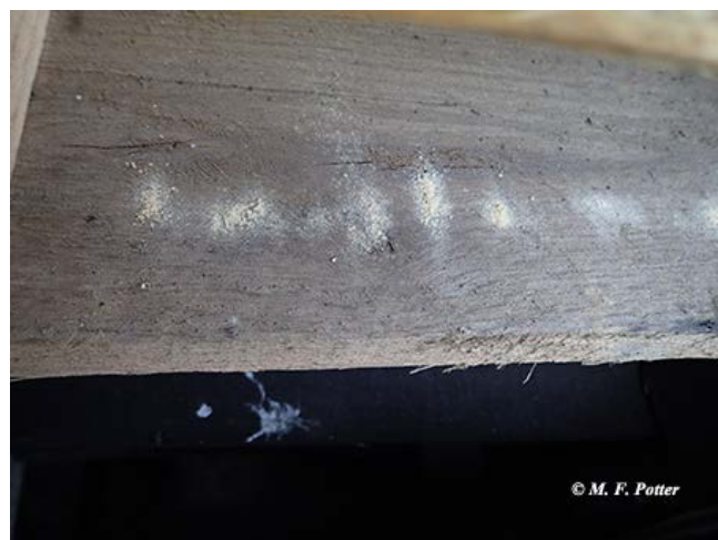
Above: Lyctid powderpost beetle near an exit hole Below: Lyctid beetle powder on a pallet
