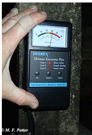
Moisture meters are useful for assessing beetle-conducive conditions
