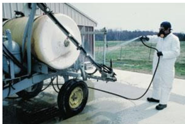
Mixing, loading, and application equipment should be cleaned and rinsed as soon as you finish a pesticide application (USDA)
